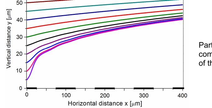
Particle trajectories computed in the vicinity of the electrodes:
