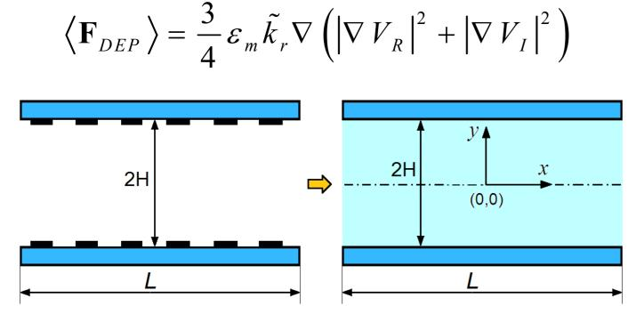
Simplified computational domain used for the concentration field calculation.
