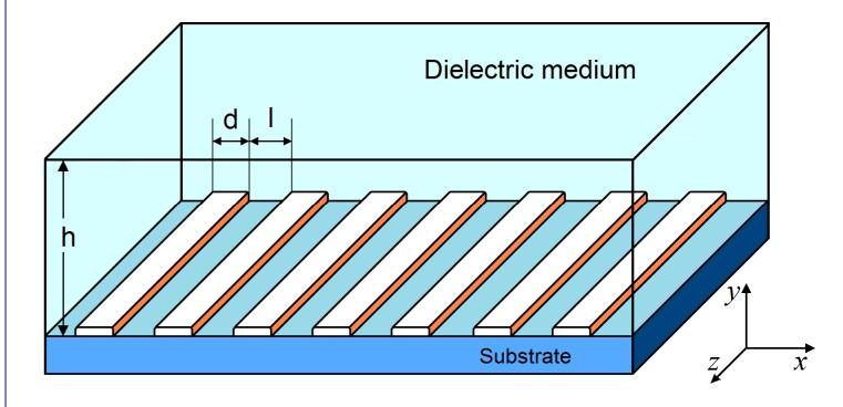
Schematic of the dielectrophoretic patterning chamber with interdigitated bar electrodes at bottom surface used for DEP separation.
