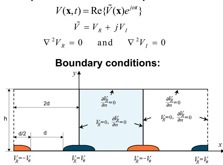
A schematic representation of computational domain with geometrical proportions and boundary conditions for the real part  $V_R$  of the electric potential. The solid lines indicate the basic unit cell.
