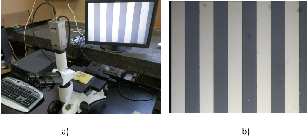
Figure 5: the installation for the analysis of the deposition plates, a), a snapshot of a detail of the deposition plate obtained at 100x, b).
