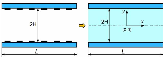
Simplified computational domain used for the concentration field calculation.
