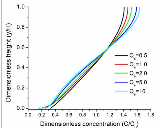
The distributions of concentration, recovered mass and particles density for different outlet width and DEP force intensities:
