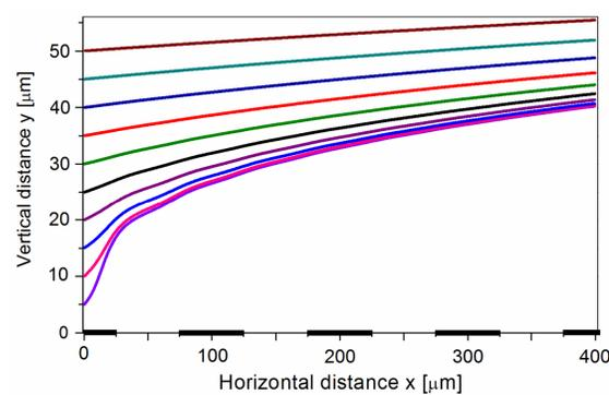
Particle trajectories computed in the vicinity of the electrodes:
