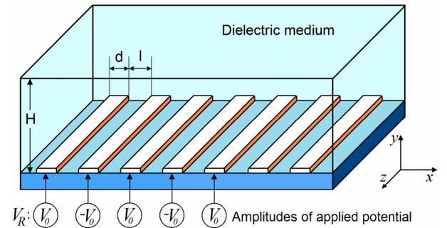
Schematic representation of the computational domain for the DEP force calculation
